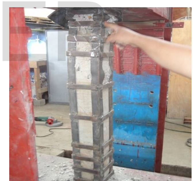
Figure (15) The failure pattern of strengthened column
